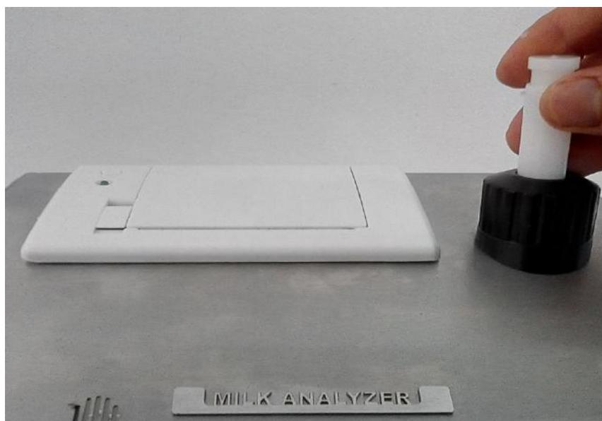
After that, put in the pH electrode and tighten the black protective cap:
