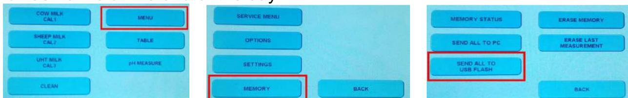
The results, saved in the flash drive are formatted in Microsoft Excel type of document and are named after the corresponding time and date of your milk analyzer Lactomat.
